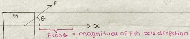
$$W = \alpha \times F = \alpha \times \text{Force in the direction of } \alpha$$
